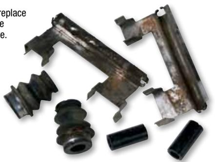
The fact is, constant tension, heat, friction and mechanical stress – the same things that caused your brake pads and shoes to wear out – will eventually cause your brake hardware to fail.
